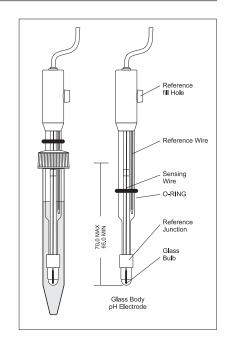
**MA9011** 3.5M KCl Electrolyte Solution. For faster response, unscrew the fill hole screw during measurements.
