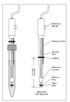
than 2<sup>1</sup>/<sub>2</sub> cm (1") below the fill hole, add **MA9011** 3.5M KCl Electrolyte Solution. For faster response, unscrew the fill hole screw during measurements.
